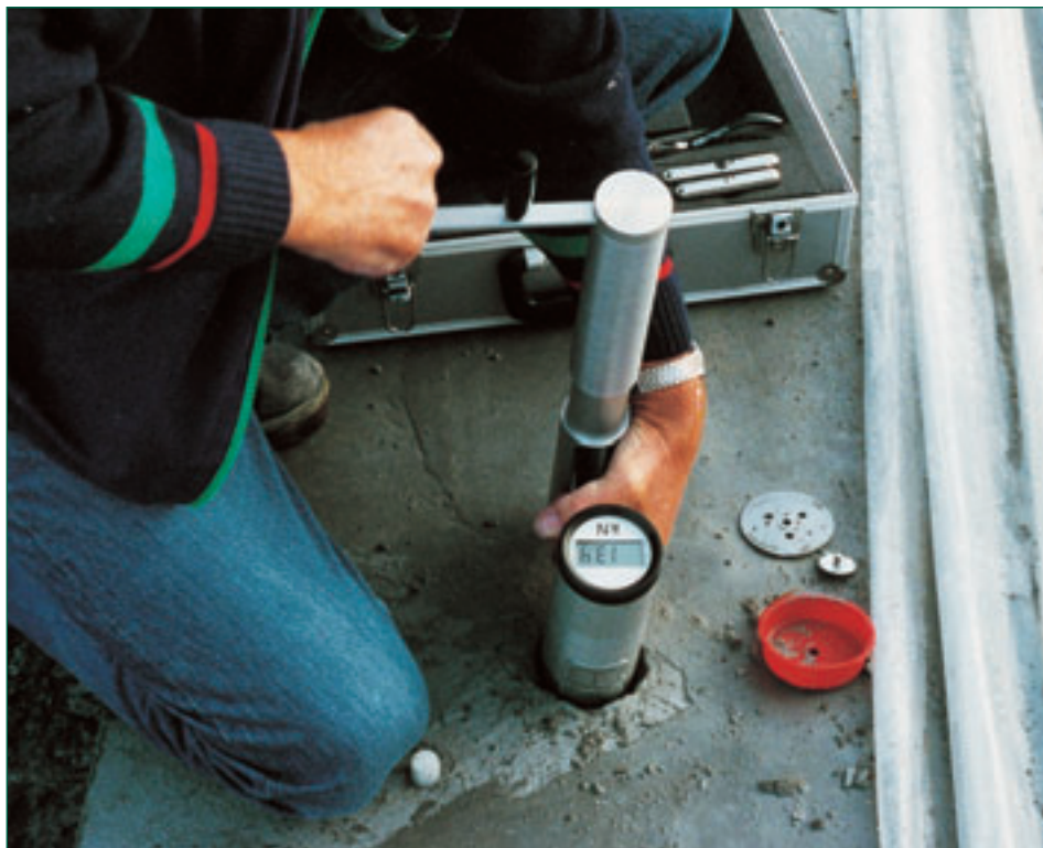
Figure 8: The Lok-test jack in position
