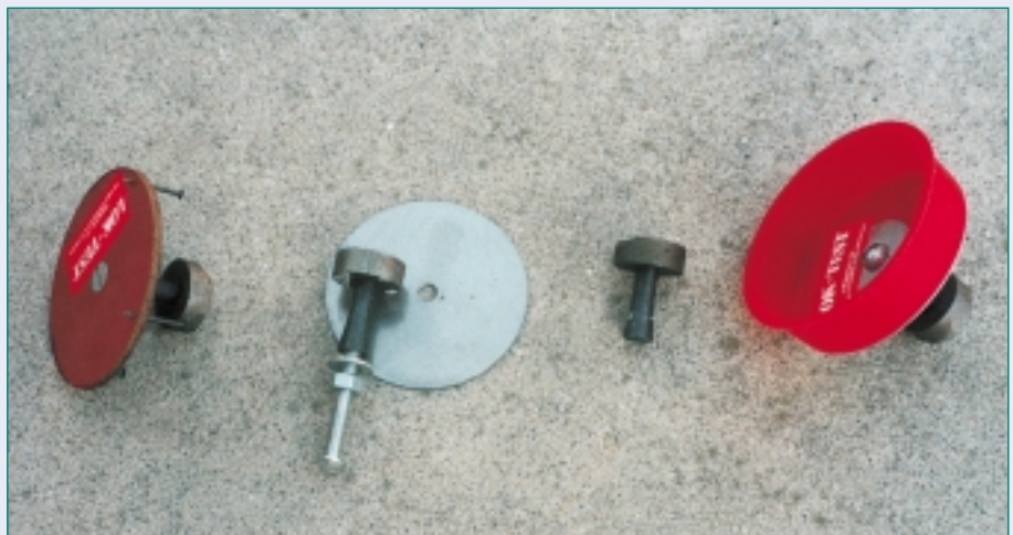
Figure 4: Lok-test inserts for formwork (left) and floating cup (right)
